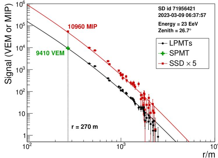
Lateral Distribution (LDF) of the signal sizes recorded in SD detectors with the help of an additional Small PMT
