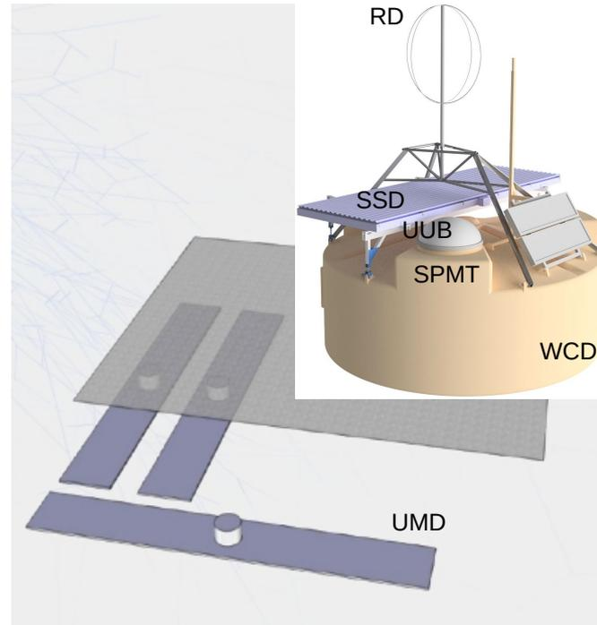
**Idea:** Use detectors with different responses to the **electromagnetic** and **muonic** air shower components.
