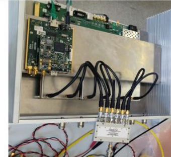
Gain characterization for the radio signal across the TAXI board with a known input signal
